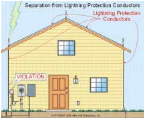
Where practicable, a separation of at least 6 feet shall be maintained between communication cables and lightning protection conductors.
