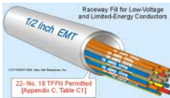
Raceway conductor fill requirements only apply when the low-voltage or limited-energy circuit require a Chapter 3 wiring method.
